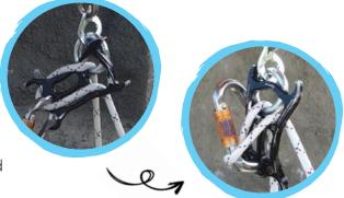
This could happen when a person is descending the rope or when the system is released and in lowering mode. Consequently, the devices braking ability could be affected or, conversely, could cause a blockage during lowering.
