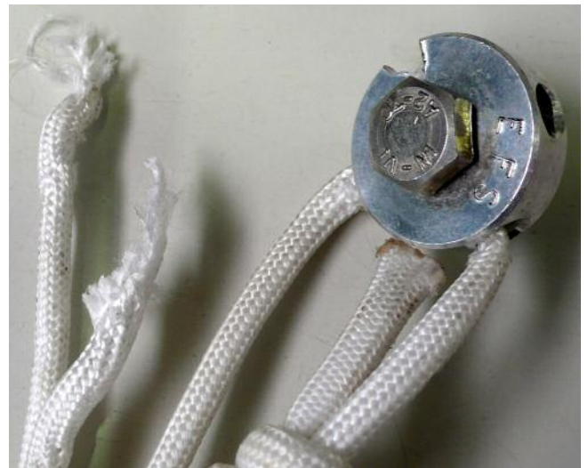
AS après rupture
